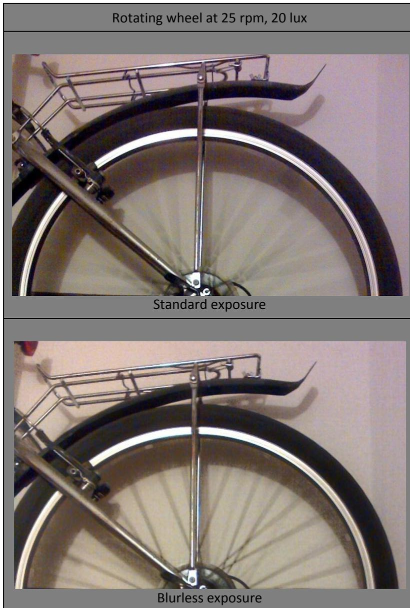
Blurless exposure is not only compensating for camera shake but also, to some degree, for motion in the scene. Better definition of the spokes is clearly visible.
