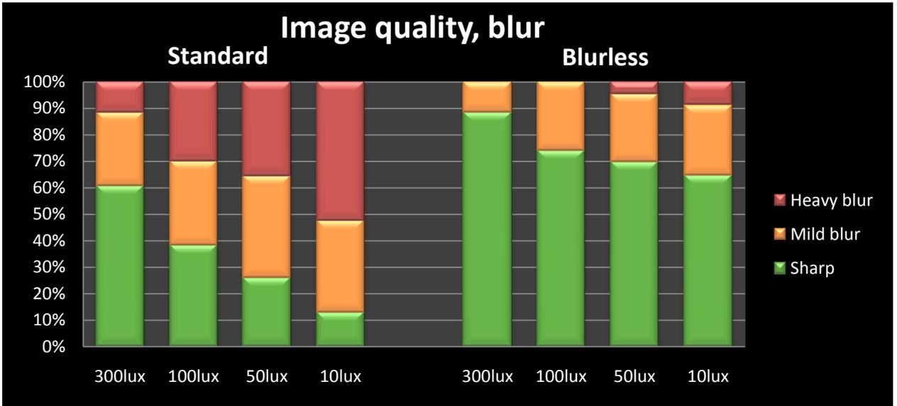
Comparison shows a great reduction in the number of blurred images versus images taken with the usual exposure method. E.g., under 100 lux illumination, less than 40% of the shots turned sharp with usual exposure, while more than 70% did so using blurless exposure, with no heavily blurred images at all.
