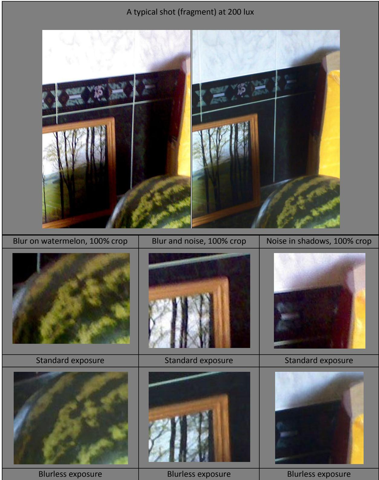
Even though average noise levels are similar, blurless exposure demonstrates a better result in shadows. An increase in dynamic range can also be seen by inspecting white tiles at the top and a dark area in the
