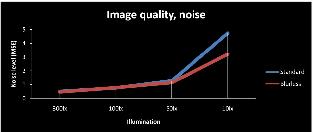
Noise levels are nearly the same at moderate illumination levels. In very low light (i.e., shadows or dark scenes), blurless exposure demonstrates significantly lower noise level.
