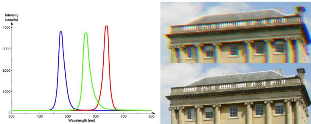
Figure 5. R/G/B-led illumination spectra<sup>6</sup> (left); displayed image without correction (top right); displayed image with correction<sup>7</sup> (bottom right).
