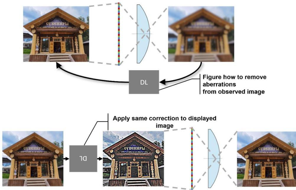
Figure 6. Schematic depiction of aberration correction method
