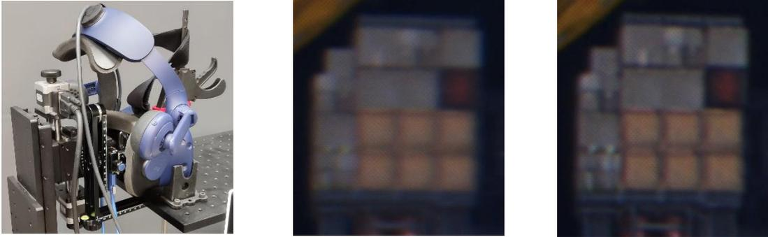
Figure 1. The Digital Lens element reliably improves the image quality of design-constrained near-eye display optical systems. From left to right: Vive Pro Eye HMD mounted for the optical measurements, displayed image with built-in correction, displayed image pre-corrected with the Digital Lens element.
